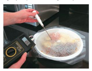
calibration). This can be done electronically, but a simple and low-cost check is to place the probe in iced water – the reading should be between  $-1^{\circ}$ C and  $+1^{\circ}$ C. To check accuracy at high temperatures, place the probe in boiling water and the reading should be between 99°C and 100°C. If probes read outside of these temperatures they need to be repaired or replaced.
